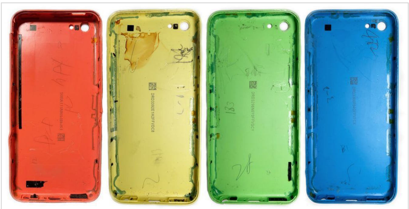
iPhone 5c cases, numbered with qr codes and with hand written batch numbers on the interior.
